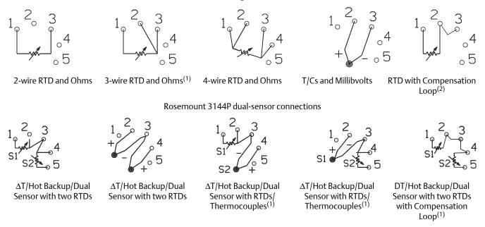
Emerson provides 4-wire sensors for all single-element RTDs. Use these RTDs in 2-wire or 3-wire configurations by leaving the unneeded leads (1) disconnected and insulated with electrical tape.
