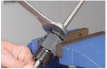
The coning tool (with the knurled cap and cutter removed) provides an ideal way to hold
