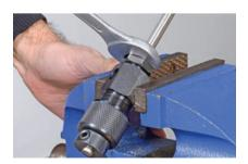
Insert tubing through collet nut and collet until tubing stops up against inside cutter. Tighten collet nut to secure tubing into position.
