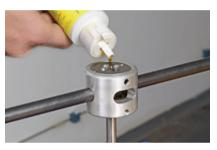
Apply a liberal amount of cutting fluid to the end of the tubing. Place the threading tool (guide bushing side first) onto the tubing.
