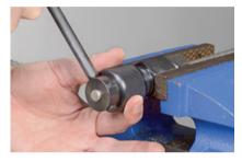
the cutter contacts the end of the tubing.
