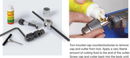
the side of the collet nut firmly with the wrench to release the collet.
