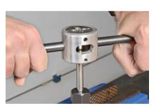
Place the palm of your hand firmly against the center of the threading tool and rotate your wrist counterclockwise. This will help "start" the die onto the tube. After you feel the die start onto the tubing, continue to rotate the threading tool using the handles. Remove the threading tool and clean off cutting fluid and chips.
