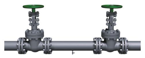
Historical double block-and-bleed system requiring the use of two valves and a spool piece. A bleed valve was used to drain the spool and verify seal integrity.
