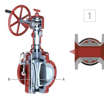
The seals (A) are permanently bonded into the slips (B), which are mounted on a central plug. In the open position, the slip seals are completely out of the flow.
