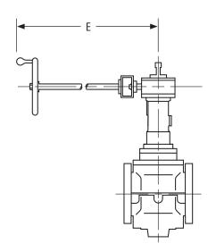
Gear operator extension lateral type C.
