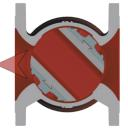
2. Turning the operator handwheel clockwise rotates the plug assembly 90° to block flow. During rotation, clearance is maintained between the seal and the valve body, enabling free movement and avoiding abrasion.
