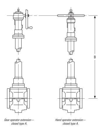
The GENERAL VALVE Twin Seal plug valve product line provides vertical and lateral extensions or combinations of the two. When ordering, specify dimension B or E.
