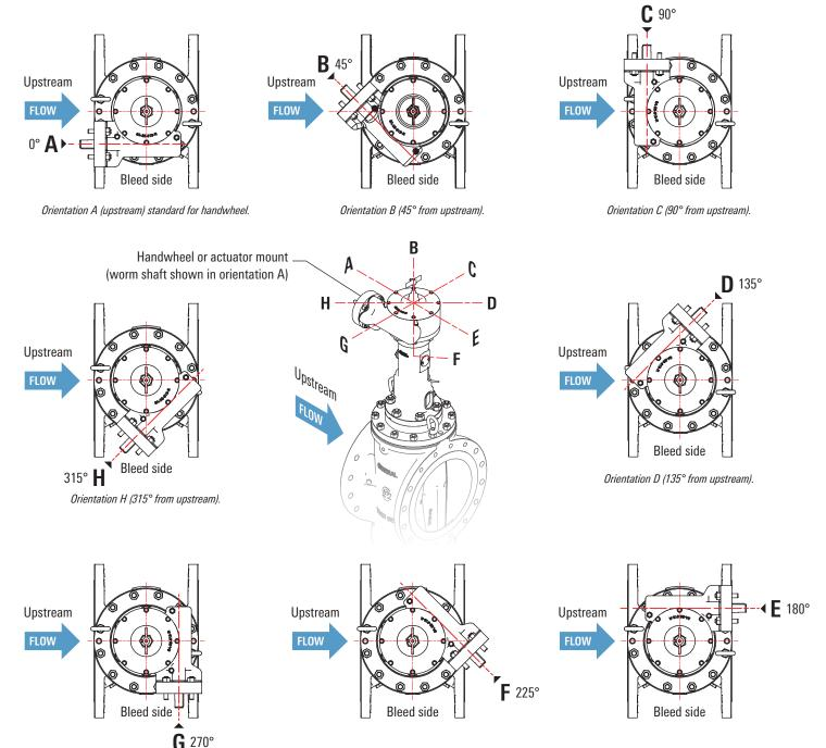
Orientation G (270° from upstream) standard for motor.
