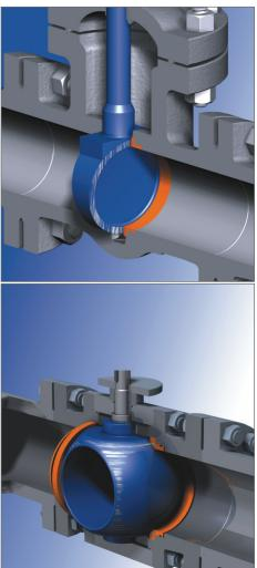
Standard gate valve design (top). Standard trunnion mounted ball valve design (bottom).
