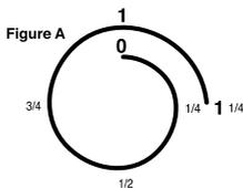
2. Tighten the nut. 1-1/4 turns of the nut is required for 1/4" (6 mm) and higher (See Figure A). 3/4 turns of the nut is required for 1/8" (See Figure B).
