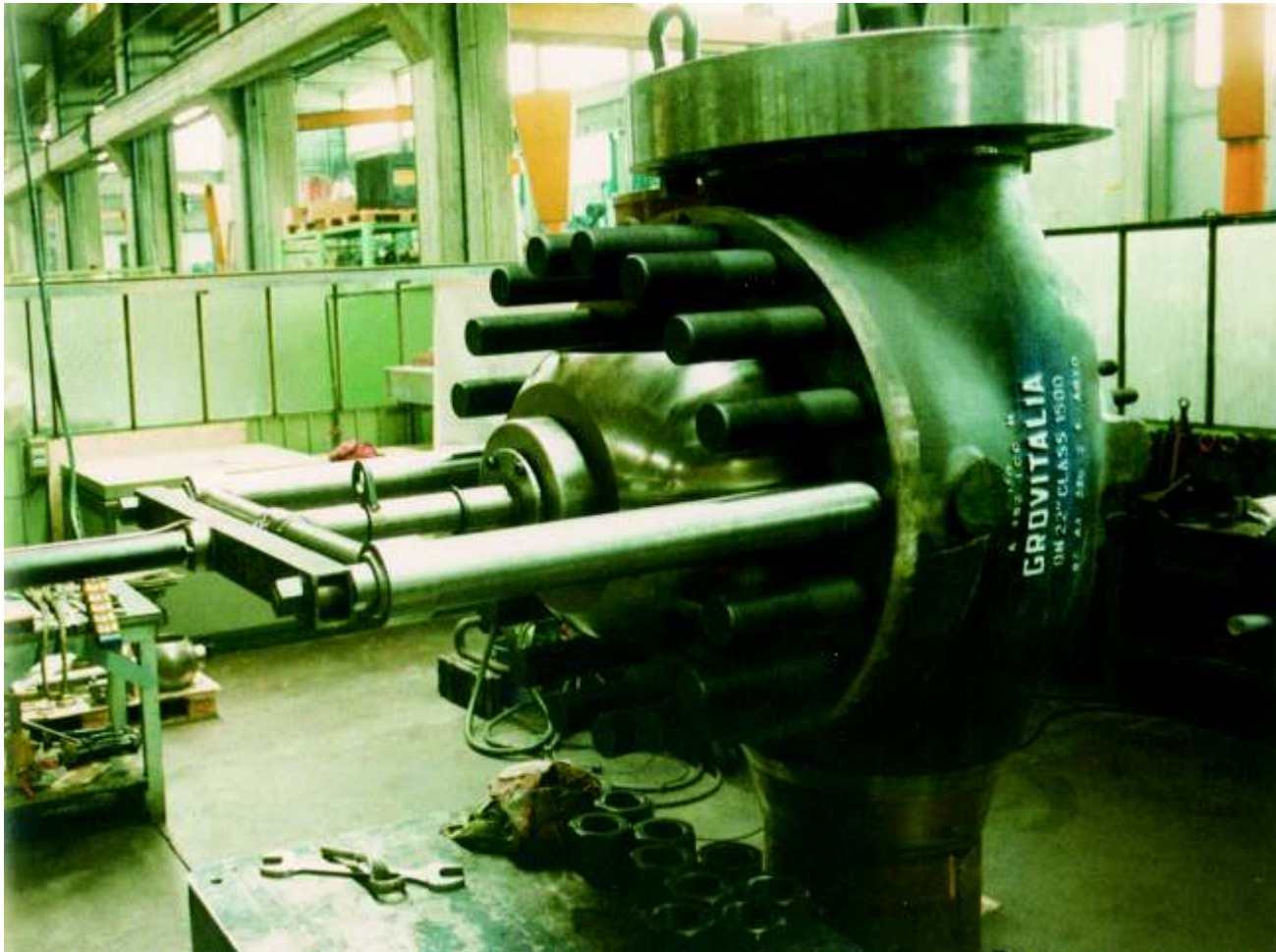
BT2 in vertical position, with special tools, during the ball assembly/disassembly operations.
